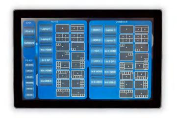
The iCON<sup>™</sup> T10W – Ten Inch Wall Mount All In One Touch Screen and Controller allows control of virtually any device. Coupled with PureLink's innovative EZ Control<sup>™</sup> platform, programming your control system has never been easier.
